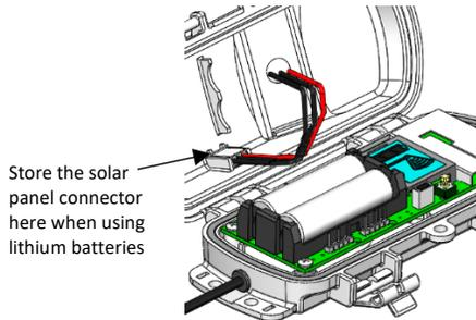
The mote contacts the network once the new batteries are installed. The green LED blinks quickly while the mote searches for a network to join and then blinks slowly while it completes the network registration. Once the mote has finished joining the network, the green LED turns off and the blue LED then blinks indefinitely while the mote is part of the network.
